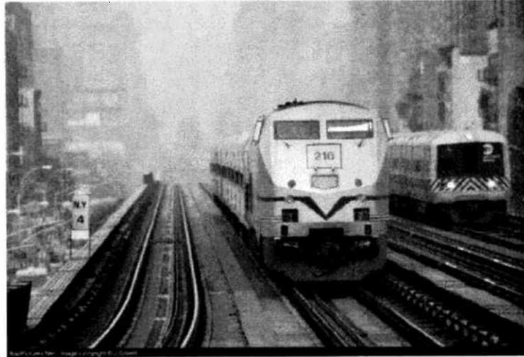
General Electric P32AC-DM operated by Amtrak. In New York City, where diesel emissions in tunnels approaching Penn Station and Grand Central Terminal are not permitted, operates on “third rail” electric power. Elsewhere, operates as a diesel-electric locomotive. Seamlessly transitions while underway. Rated at 3,200 hp (2,390 kW) and can obtain a maximum speed of 110 mph.
